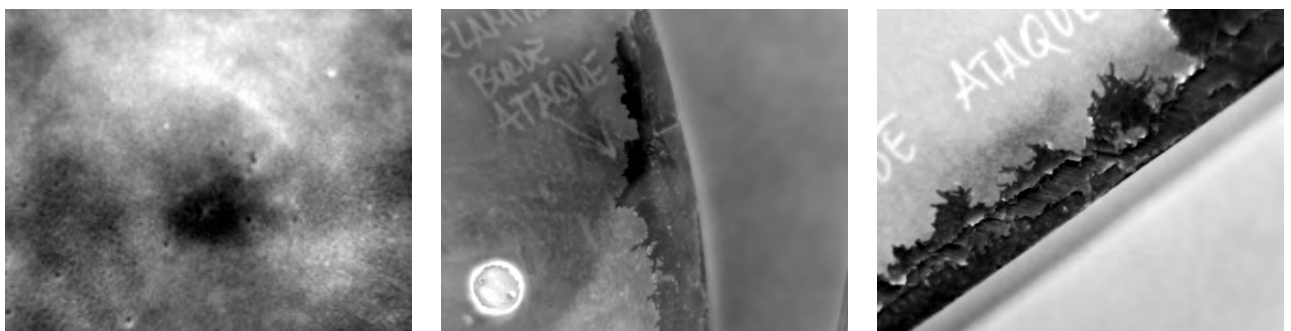
Impact delamination FFT 0,012 Hz (left), leading edge delamination, FFT 0,018 Hz (center) and leading edge erosion FFT 0,012 Hz (right). (LORTEK)
